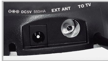
1- Power connection: DC Connect the AC adapter to the DC5V/550mA jack at the back of the antenna and plug the AC adapter into a standard AC outlet.
