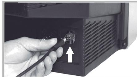
2- Connect to TV: Connect the end of the coaxial cable to the TV's RF input socket.
