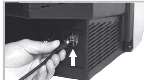
2- Connect to TV: Connect the end of the coaxial cable to the TV's RF input socket.
