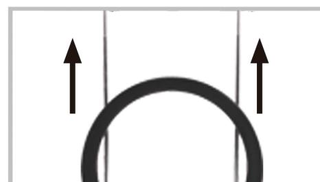
4- Antenna adjustment: When receiving UHF signal (470-790 MHz), adjust the loop to the best reception angle. When receiving VHF signal (174-230MHz), extend and move the dipoles to the best reception.
