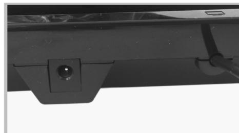
1- Power connection: DC Connect the AC adapter to the DC5V/550mA jack at the back of the antenna and plug the AC adapter into a standard AC outlet.
